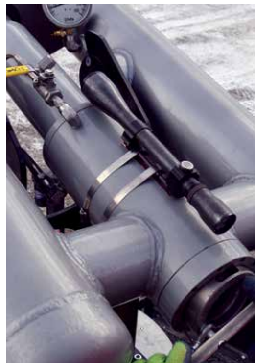
Rifle scope for precise backsighting. Photo Courtesy Alaska DOT
