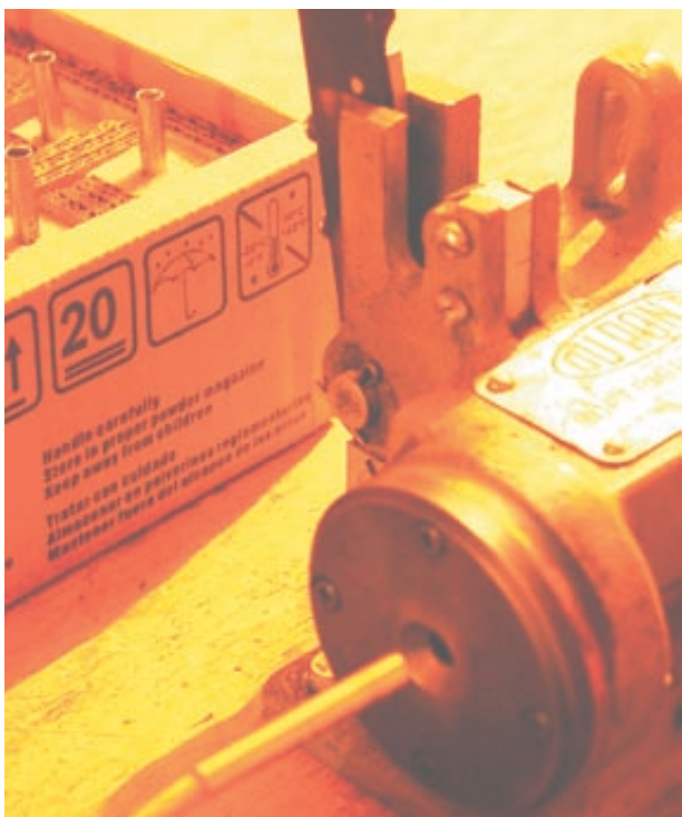
A venerable DuPont bench crimper at work. These units are no longer manufactured. Photo by John Brennan
