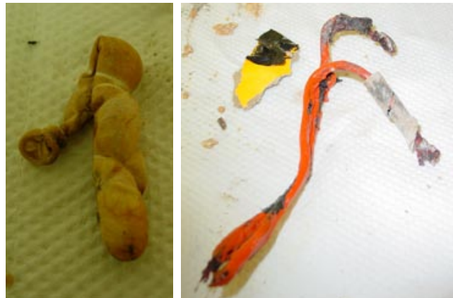
Left: The balloon that contains the sensitizing compound for the bulk of the cast shot was found about 30 feet from the blast crater. Notice the striations left from the rubber band.
